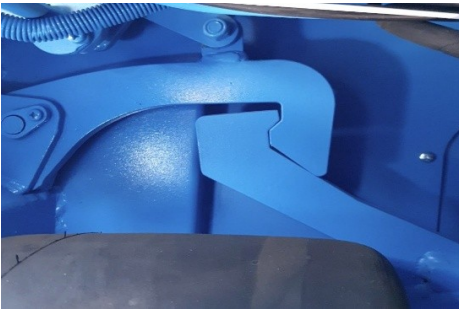
Figure 36. Locking the locking tongue to the axle to lift the axle.
