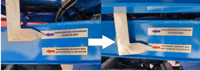
Figure 24. Camelback level indicator. Adjusting from driving position to unloading position.
