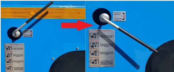
Figure 33. Moving the axle lock lever from the loading/unloading position to the driving position
