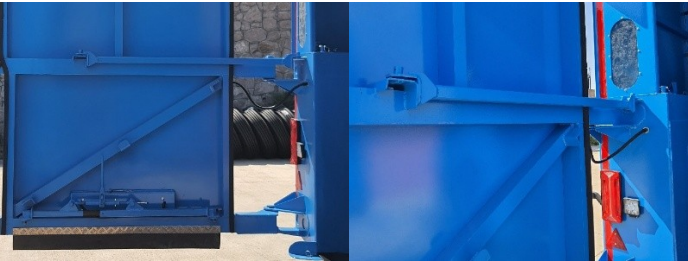
Figure 28. 90° door opening and securing with the top arm
